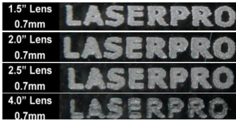
Engraving effects achieved with the different lenses
